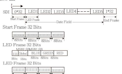
Global bit: 5-bit (32 level) brightness setting, while controlling R, G, B three-color constant current output value, if set the Global bit for the 10000 (16/31) is the output current is half again the original PWM settings.
