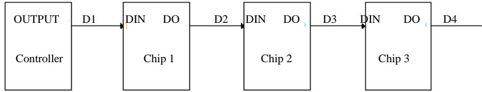
D1 is the datum transmitted by controller, D2,D3,D4 are the data retransmitted by cascade TM1829.
