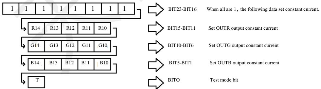
RI [bit15~bit11]:Set R channel constant-current value,  $I_r=10+RI[4:0]mA$ , namely minimum  $10+0=10mA$ , maximum  $10+31=41mA$
