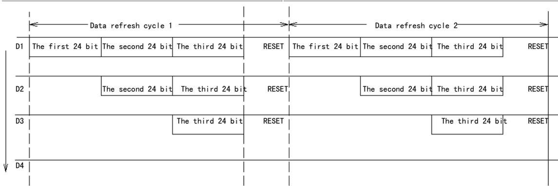
Chip cascade, data transmission and retransmission procedure: Data (D1) is sent from controller. When chip 1 finishes receiving the first 24bit, chip 1 does not retransmit data (D2) still and controller continues to send data, chip 1 receives the second 24bit. As the first 24 bit is existed in chip1, chip 1 retransmits the second 24bit out through DO.
