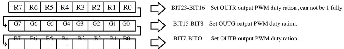
PWM duty ration can be regulated from 0 to255 continuously. Attention: high 8 bits are not 1 in full.
