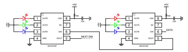
5V application, few peripheral components, transmission distance between two points can be 30m.
