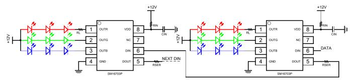
12V application, a 180ohmic resistor  $R_{SER}$  is recommended to cascaded at the signal output port to avoid the damage of the IC input port caused by the inverse connection between the electric plug and the signal line or between the power supply and signal line, the transmission distance between the two points of the 180ohmic resistor  $R_{SER}$  can be 10m.
