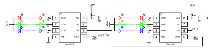
24V application, a 470ohmic resistor  $R_{SER}$  is recommended to cascaded at the signal output port to avoid the damage of the IC input port caused by the inverse connection between the electric plug and the signal line or between the power supply and signal line, the transmission distance between the two points of the 470ohmic resistor  $R_{SER}$  can be 5m.
